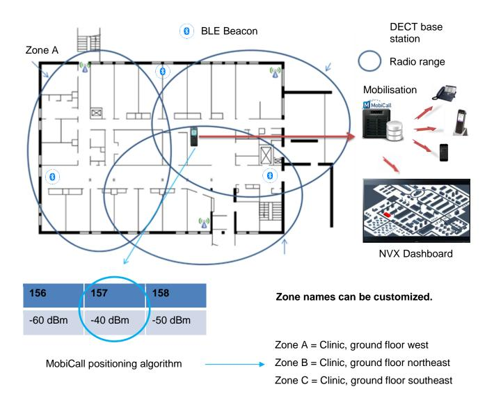
Based on your ALE DECT infrastructure, emergency calls can be triggered via DECT devices and located with floor accuracy. The DECT device that triggers the alarm detects the DECT antenna(s) and MobiCall uses this information to calculate the location.
